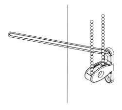
Attach the cord cover plate with the screw provided.
