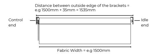
Use this figure to position the outside of your brackets accordingly whether inside of the recess or outside of the recess
