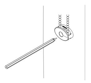
Split the cord tidy and mark the remaining offset hole position before drilling and plugging both location holes if necessary. Screw into the offset hole to fix the back piece of the cord tidy to the wall.
