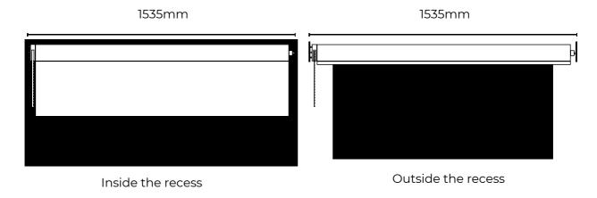
Mark the hole positions before drilling and plugging if necessary. Use two screws in each bracket ensuring that the brackets are level. Remember to allow room for the blind to clear any obstacles when deployed, e.g. door or window handles.
