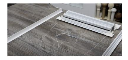
Select the left hand frame component and guide onto the exposed arm of the bottom left corner joint.
