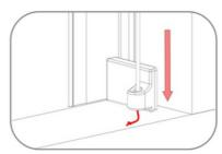
11. If your blind requires further tension pull the cord through the hole in bottom button until you feel the blind has sufficient tension and tie a fresh knot.
