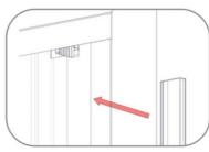
5. Place the flat side of the side extrusion against the glass with the notch to the bottom.
