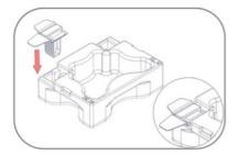
Place the top corner bracket into the slot on the fitting tool.
