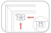
2. Position bracket behind the rubber bead and carefully push until the metal legs are behind the rubber bead.
