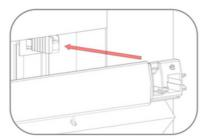
8. Align headrail endcaps with top corner fixing brackets and push fully home.
