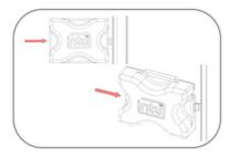
7. At the appropriate position(s) on each side profile, fit retention clips (long side profiles only). Press into position using the fitting tool.
