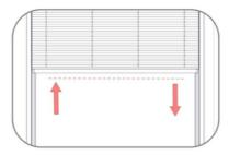
10. To align the bottom rail horizontally, simply pull it into the position desired. It will stay in position under tension from the cords.
