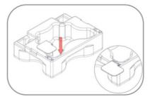
3. Check bracket is square to the sides of the bead and it is secure. Repeat for other side. Place the bottom corner bracket into the slot on the fitting tool.
