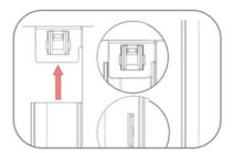
6. Slide the side extrusion up until it slots into the top corner fixing bracket. The side extrusion should rest under the bracket. Push the slot at the base of the extrusion over the bottom corner bracket. Repeat for both sides.
