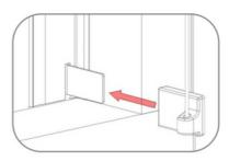
9. Align bottom button with bottom corner brackets. Slide the bottom button onto the bracket until it locates. Repeat both sides
