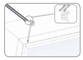
1. Position brackets a minimum of 12mm from the front of the recess, mark through centre hole. Ensure brackets are not fitted directly above internal components as this can impede the rotation of the cord drums which will impact operation of the blind.
