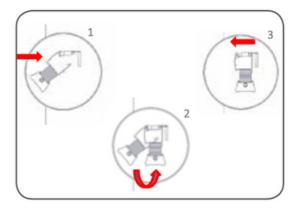
4. Fit blind to brackets by first locating front ledge on plastic part of bracket (1), then compress springs by pushing rail away from you as back edge of rail is rotated up towards brackets (2). Once flush against brackets rail should release to engage back ledge on brackets (3).
