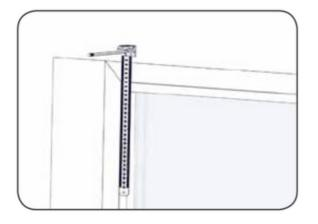
1. Position bracket on face at a height where measurement has been taken from. Mark through 2 x holes in bracket (using centre slot allows some adjustment). Ensure brackets are not fitted directly above internal components as this can impede the rotation of the cord drums which will impact operation of the blind.
