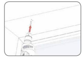
2. Using your mark as a guide. Drill into the frame. Repeat this process for all brackets.
